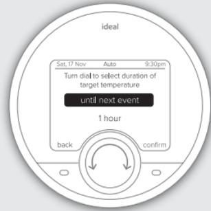
Turn the dial to select how long you would like the target temperature altered for. You can select either until the next change in heating temperature is scheduled or a number of hours.
