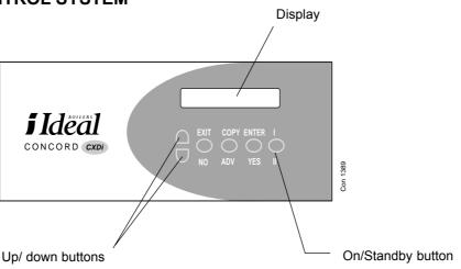
The **CXDi/H** incorporates an advanced microprocessor based control system which operates all electrical functions of the boiler, including automatic ignition, flame detection, thermostatic control and high/low burner operation. In addition, the microprocessor also has onboard commissioning and servicing instructions and a fault diagnosis programme.
