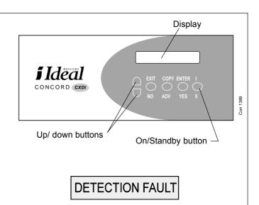
In this case, the ignition sequence should be reset by pressing the [COPY] button.
