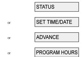
To select any of the above, use the [UP] or [DOWN] button until the option required is displayed and press [ENTER].
