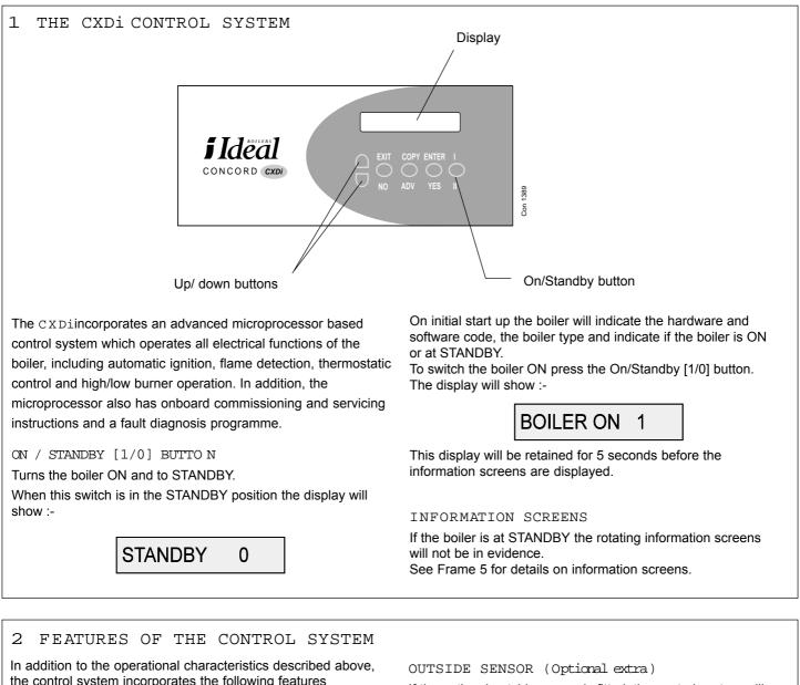
the control system incorporates the following features accessible to the user or service engineer:
