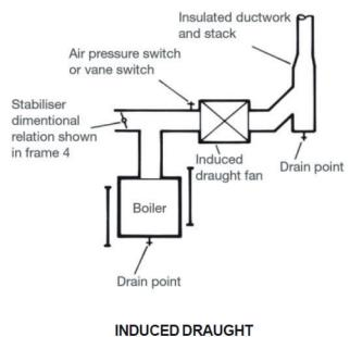
**Note**: Air intake and discharge should be on the same outside wall face. Design must comply with British Gas requirements - refer page 5 and Publication IM/11.
