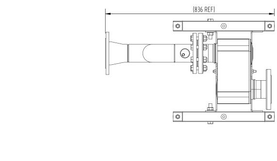
Note 1: Plate Heat Exchanger and gas connections can be located either on the LHS or RHS of the assembly to suit the needs of each particular system.
