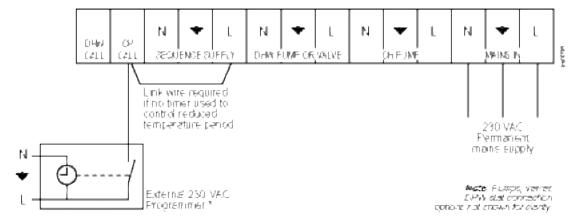
\* The swhched live from external controls must be from the same phase supply as the boller mains supply to ensure that when the boller supply is swhched off the controls are also isolated.
