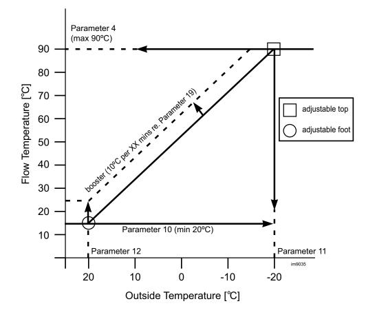
purpose of the booster function is to increase the set flow temperature by 10°C for every XX minutes the thermostat remains closed (where XX minutes = parameter 19) this value is factory limited to 90°C. Once the thermostat contacts have opened, the set flow temperature will decrease by 1°C for every minute of open contacts.
