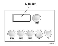
Code Mode is entered from standby mode by pressing and holding the 'mode' and 'step' buttons.
