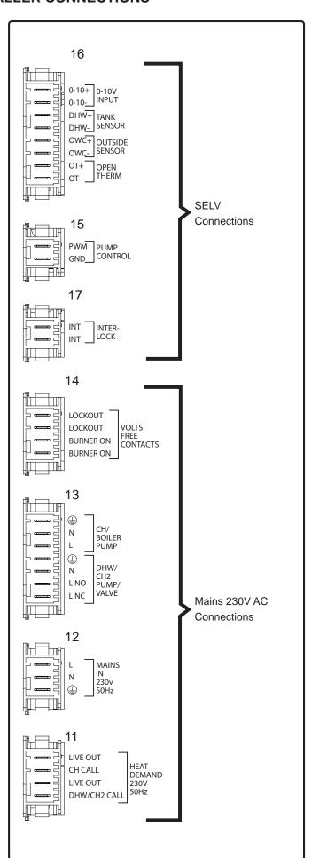
If a Pump is to be run directly from the boiler and the electrical current draw is 1.3A inductive or less then the pump can be connected directly into the CH Pump or DHW Pump connections, as appropriate. If the current draw is more than this then an external relay or contactor should be operated by the CH Pump or DHW Pump connection, with the external contact then powering the pump.
