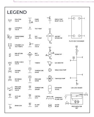
Note: this schematic is an illustration of a hydraulic arrangement for discussion and reference use only.
