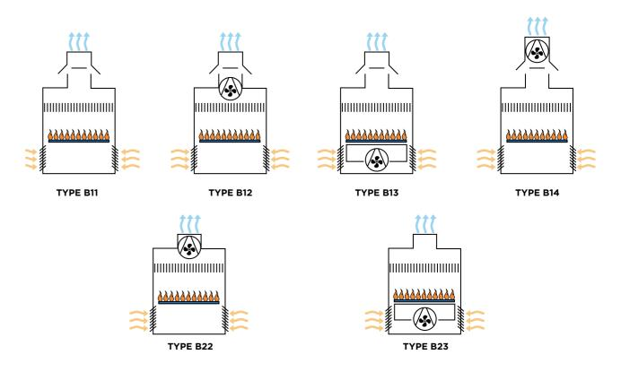
Where 2 or more gas fired boilers are connected to a common natural draught flue, the boilers must be installed in the same room and have the same type of burner system. A gas fired boiler and a solid fuel or biomass boiler must not discharge into the same flue. A gas fired boiler and a liquid fired fuel boiler can discharge into the same flue providing they are both installed in the same room and are force draught.
