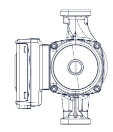
Note: pumps with screwed connections are G1.1/2" x 180mm.
