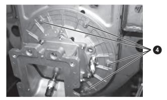
5. Remove the five screws retaining the fan mounting manifold and remove the manifold.
