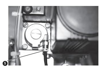
6. Remove the four socket cap screws retaining the gas valve to the outlet flange.
