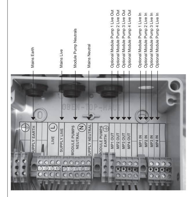
Connection 2: Inside Master PCB Box (top, right hand side of Master Module)
