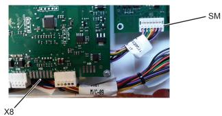
4. Fit the interconnecting lead between the X8 connection on the KM821-i5 PCB X8 and the KM connection on the TTL-i5 PCB.
