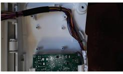
2. Locate and fit the TTL-i5 adapter PCB and secure using the two screws provided into the location on the RHS of the facia.
