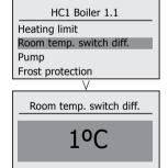
iv. Pump - The heating circuit pump overrun time can be set here. If the heating circuit pump is controlled by 0-10V then additional speed parameters can be set.
