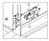
remove the nuts (4) that secure the hinge plate (5) to the door and remove the plate.
