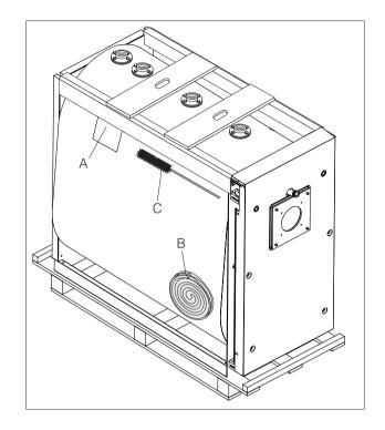
2) PANELLING CRATE, complete with assembly accessories, protected by cardboard packaging and a wooden crate.
