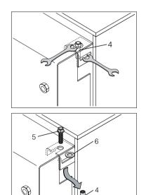
nsert a spanner through the top slot and hold the bushing (4) steady. Unscrew the top bolt (5), then remove the bushing (4) and washer (6).
