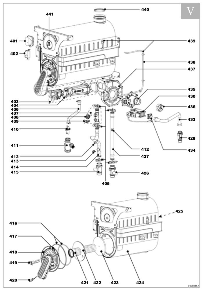
figure 37 - Body and burner for EVO S 135 model
