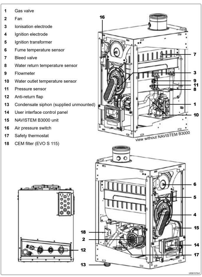
figure 3 - Boiler components for EVO S 70 to EVO S 115 models
