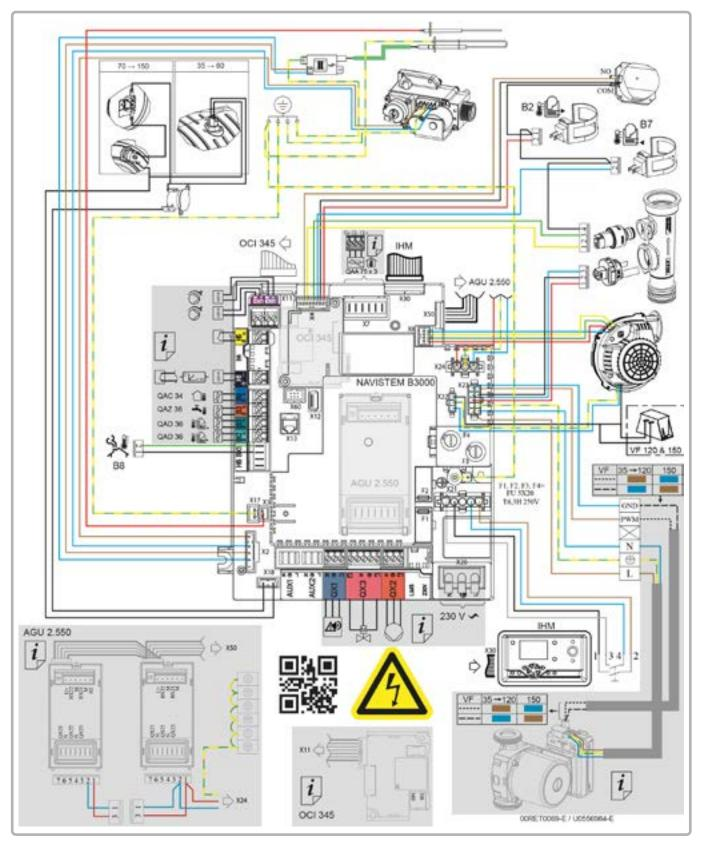
figure 17 - Wiring diagram
