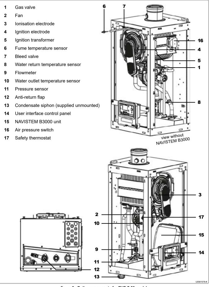
figure 2 - Boiler components for EVO S 50 model
