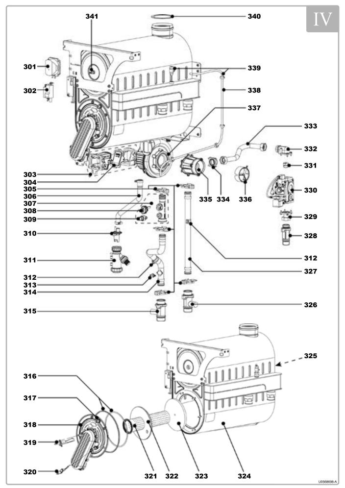
figure 36 - Body and burner for EVO S 70 to 115 models
