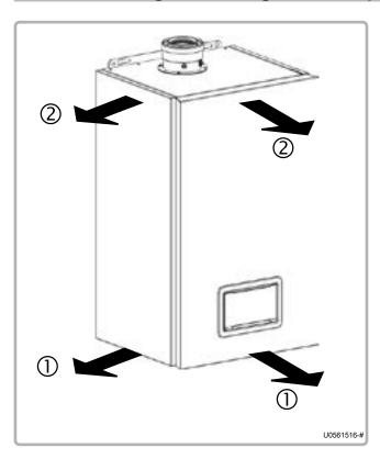
figure 6 - Removing the trim doors
