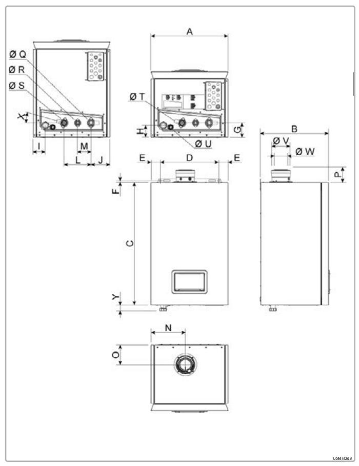
figure 1 - Dimensional characteristics
