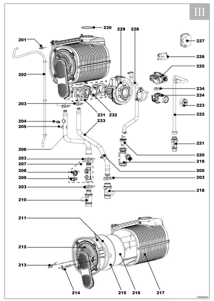
figure 35 - Body and burner for EVO S 50 model
