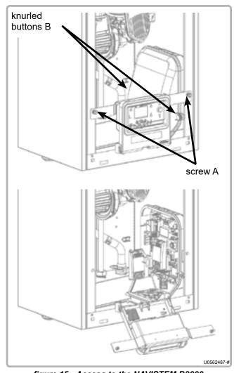
figure 15 - Access to the NAVISTEM B3000
