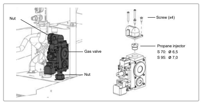
figure 10 - Installing the propane injector
