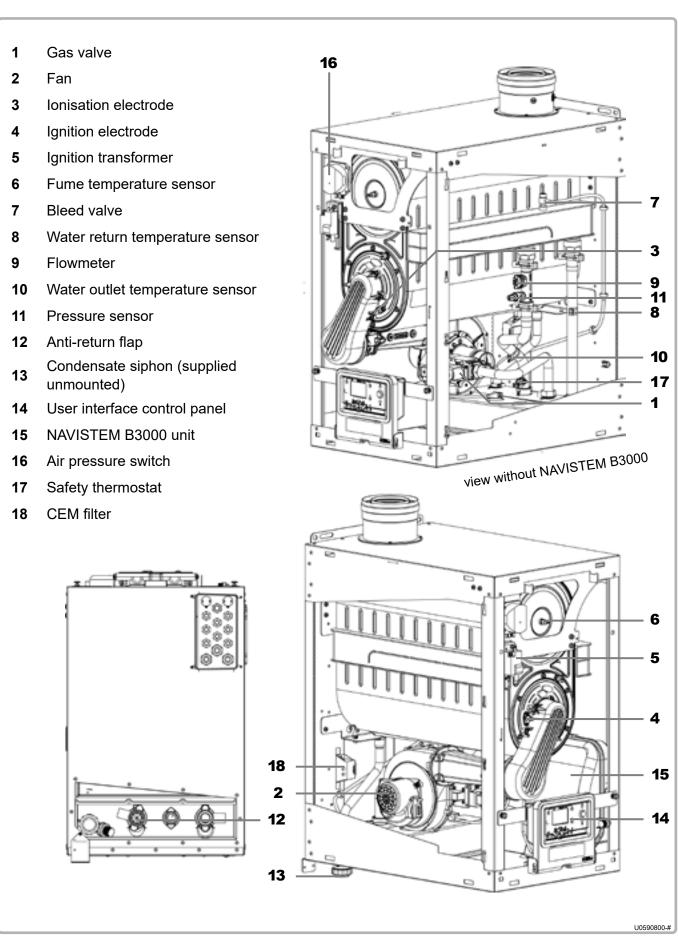
figure 4 - Boiler components for EVO S 135 model
