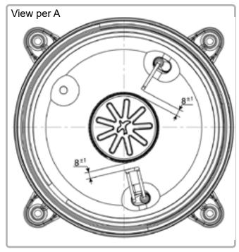
figure 20 - Position of the burner electrodes
