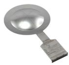
Burst Discs consist of a thin membrane which is designed to break and open when the specific level of differential pressure rises above the resistance limit that the disc was originally calibrated for, so as to allow for the excess pressure to vent out safely.
