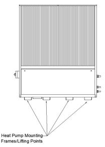
**NOTE:** Refer to latest product drawings for dimensions of mounting frames and lifting points.
