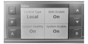
To change the control type press ENTER and DOWN key simultaneously to access the menu:
