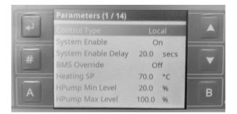
Press ENTER, then using UP/DOWN keys, scroll through to the correct control type.
