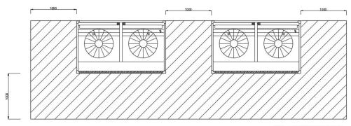
Note. 1 Meter to be kept clear to allow access to heat pump, shown in hatched region.
