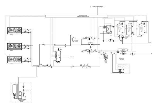
**NOTE:** Consideration will need to be made to system volume in this configuration. Dependent on control and storage of DHW store a buffer on the primary system may be required.
