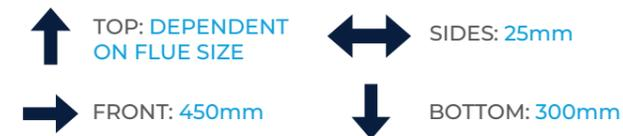
CLEARANCE BETWEEN MULTIPLE BOILER INSTALLATIONS: 25mm
